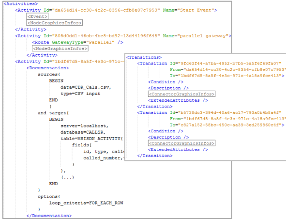
Fig. 5. A XPD XML excerpt used for the serialization of a BPMN process (Fig. 4)
