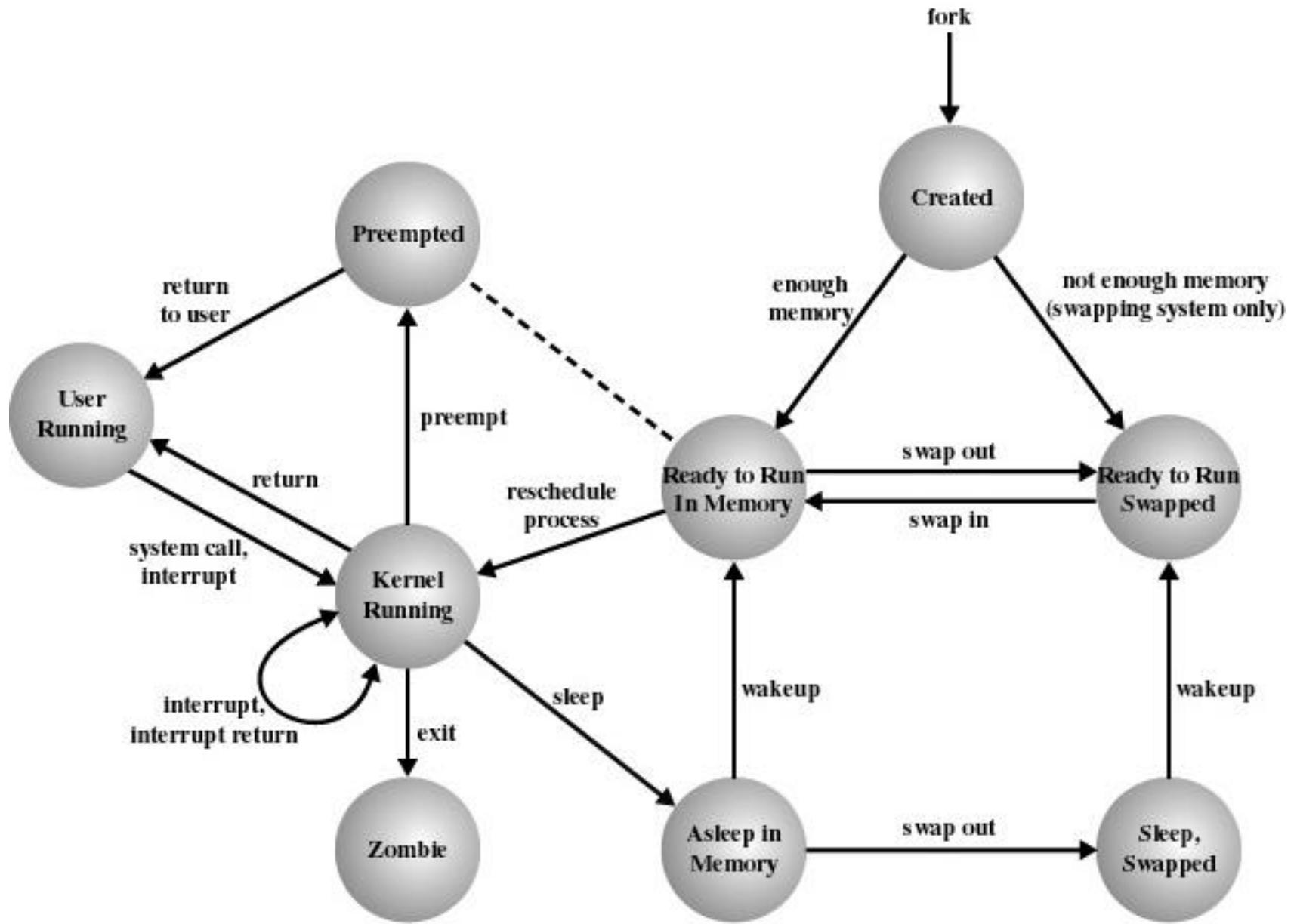
Figure 3.16 UNIX Process State Transition Diagram
